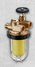
Heating oil **filters Oilpur** are used in oil firing systems that are operated as one pipe system with or without return flow feed or as two pipe systems. Filters with **plastic filter cups** are generally only approved **for suction operation**. **Metal filter cups and the filter cartridge** are also approved for **pressurised systems** and are available optionally or as accessories.
