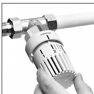
Photo 11: The handgrip now is to be replaced so that figure "2" is in line with the indicator mark. The setting is now blocked in position "2" (approx. 16 °C). Push down handgrip with hand firmly to secure.
