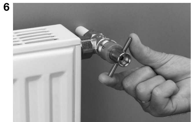
Presetting is carried out by turning anticlockwise (one complete turn corresponds to presetting 1 etc., max. of 6 turns).
