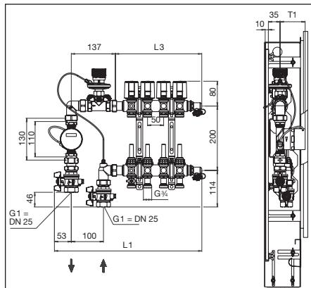
Illustr. 2 Example: Heat meter connection set, angle pattern and stainless steel distributor/collector "Multidis SF" for surface heating systems, lengths and depth
