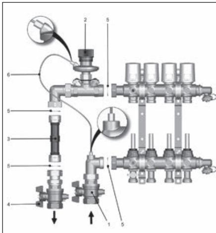
Illustr. 4: Heat meter connection set, angle pattern, extent of supply and location of the components for left hand side connection
