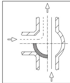
Mixing of the volume flow is achieved by a rotation of the spindle of the mixing valve.
