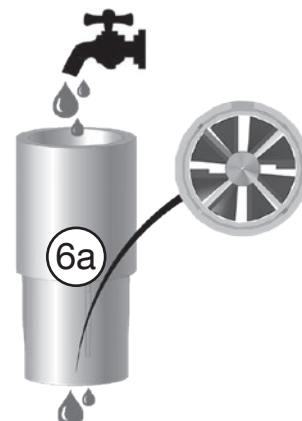
Illustr. 5.18: Clean the measuring turbine under running water
