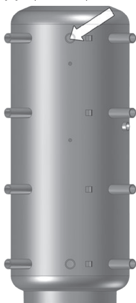
Illustr. 4.7: Position for the connection of the “storage cylinder circuit - supply” pipe of the fresh water station to the buffer storage cylinder
