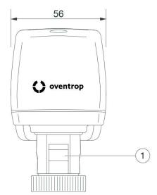
(1) Push button for releasing the engaged valve spindle
