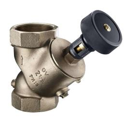
Double regulating valve for static hydronic balancing of pipe networks in closed heating and cooling systems. It offers a measuring function via the valve seat, which is, however, closed with a blind plug when delivered.
