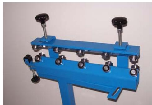
Adjust upper roller rail (5) with the help of the adjusting screws (2) to suit the corresponding pipe diameter.
