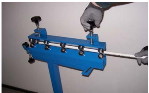
Feed the pipe into the roller bearings of the pipe straightener until it is completely inserted. Tighten the adjusting screws (2) until the roller bearings slightly touch the pipe. Do not overtighten in order to avoid damage to the pipe.
