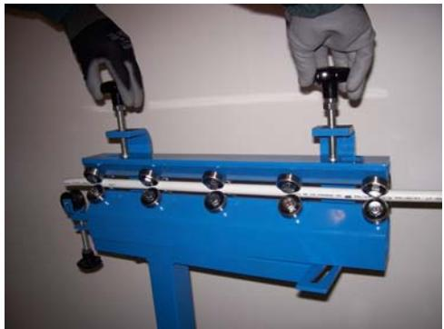
If the pipe is still bent after having straightened it for the first time, apply more pressure with the pressure roller (3) by using the adjusting screws, then re-pass the pipe through the rollers.
