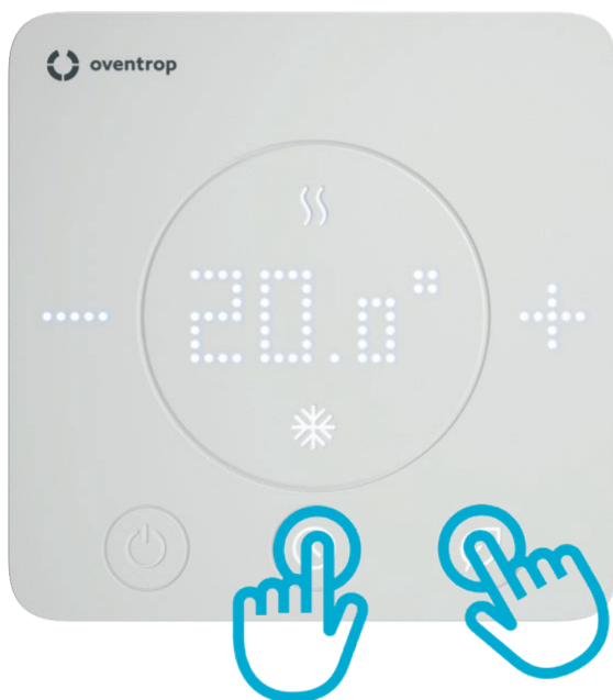
Fig. 11: ClimaCon F - Activation of the teach-in mode
