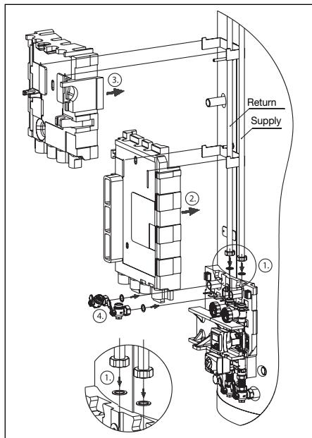
Illstr. 11 Installation of thermal insulations
