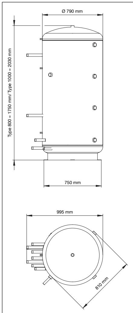
Illustr. 42 Dimensions of storage cylinder without insulation
