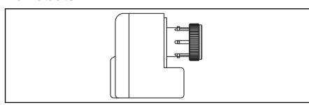
Illustr. 52 Actuator for the activation of a three-way valve (101 27 10).
