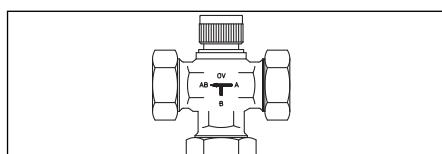
Illustr. 50 Three-way valve for two-zone loading (113 17 06).
