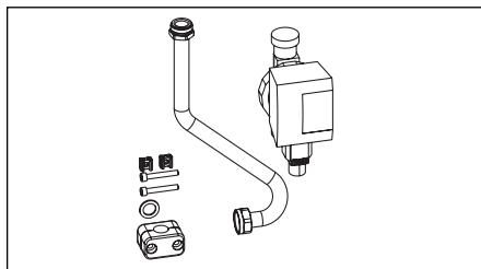
Illustr. 45 Connection set with circulation pump Wilo Star Z Nova C and time switch for the extension of the portable water station "Regumaq XH" by a portable water circulation (138 10 47 **with** circulation pump, 138 10 49 **without** circulation pump).
