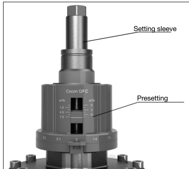
Illustr. 2 Setting sleeve (must be unscrewed before modification of the presetting)
