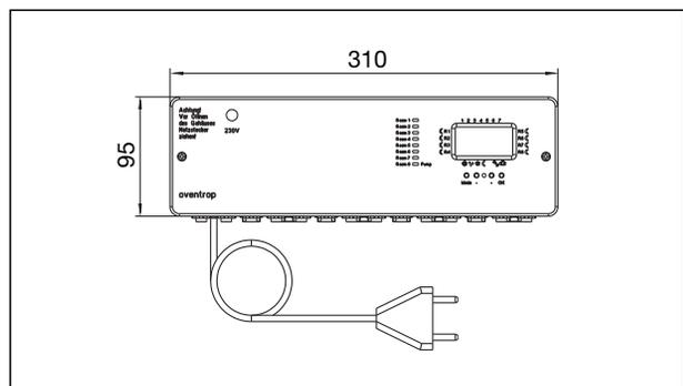
Dimensions wireless receiver with time switch, 8 channels
