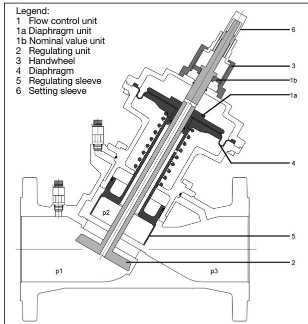
Illus. 5 Construction of the "Cocon QFC/QGC" valve
