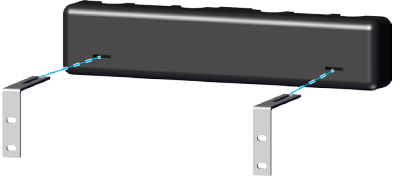
Fig. 4: Position of the wall brackets
