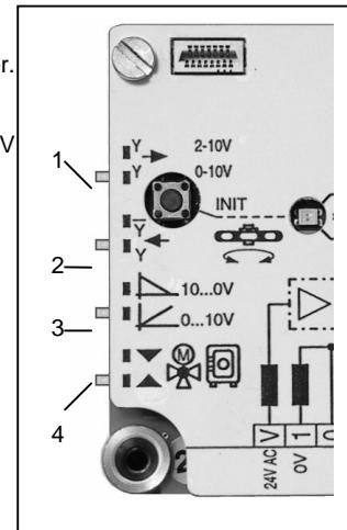
(4) **Switch:** Setting of the actuating direction for partial initialization.
