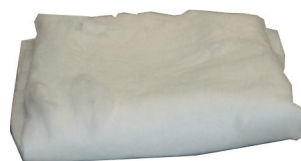
Fleece for storage cylinder coating
