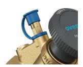
Every HydroCom A is fitted with a HydroPort auxiliary valve as standard. The HydroPort allows snap on connection of accessories. The HydroPort is opened by turning anti clockwise with an open ended 8mm spanner. For pressure pickup (impulse tube connection) one quarter of a turn is sufficient. For draining, filling and venting full flow capacity is reached after one full turn. The HydroPort has a Kvs-value of 0.3.
