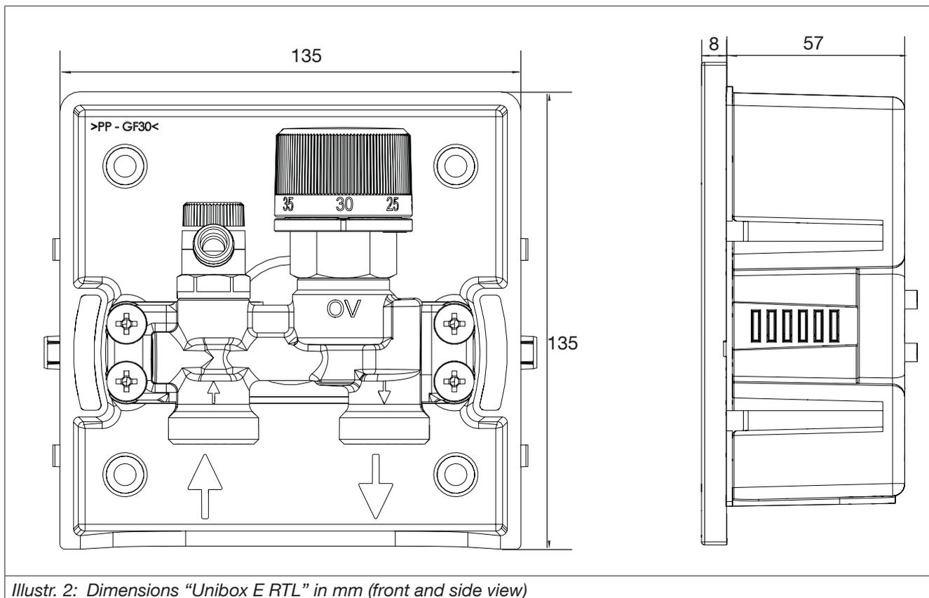
Illustr. 2: Dimensions “Unibox E RTL” in mm (front and side view)
