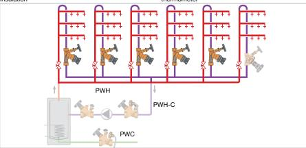
Circulation system with "Aquastrom VT" and "Aquastrom C"
