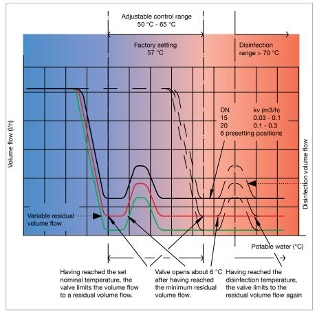
Functional scheme and characteristic lines "Aquastrom VT"
