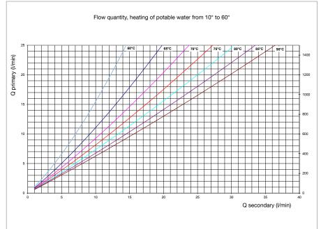
Draw off capacities (Q secondary) of the "Regumaq X-25" station depending on the buffer storage cylinder temperature
