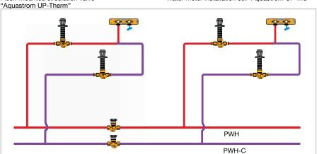
System illustration flush-mounted valves "Aquastrom"
