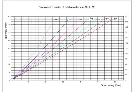
Draw off capacities (Q secondary) of the "Regumaq X-45" station depending on the buffer storage cylinder temperature
