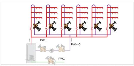
Circulation system hydronically balanced with the help of double regulating and commissioning valves
