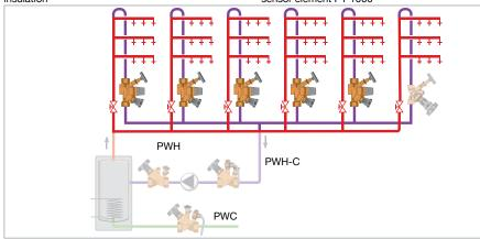
Circulation system with "Aquastrom T plus" and "Aquastrom C"
