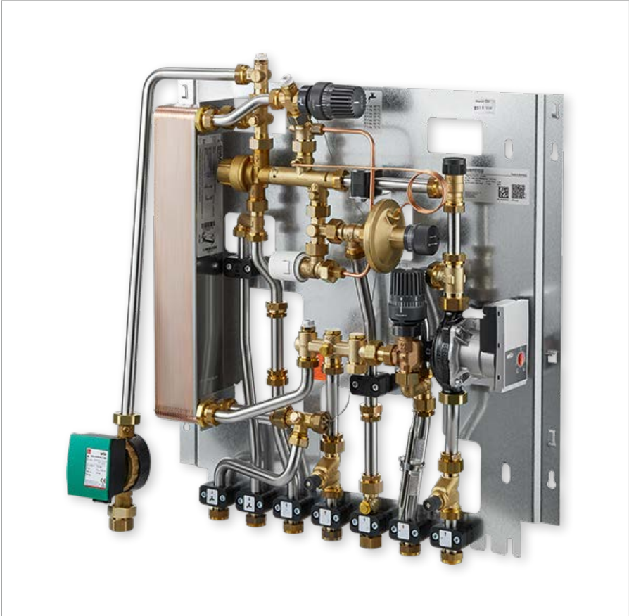
“Regudis W-HTF” with variable temperature heating circuit, circulation pipe and additional outlet for a radiator circuit and a time controlled potable water circulation pipe
