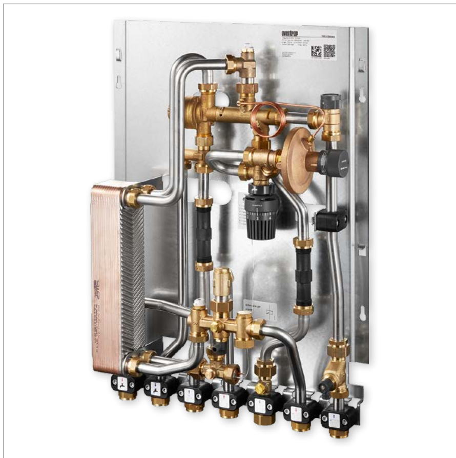
Dwelling station "Regudis W-HTU" with plate heat exchanger for the transmission of heat from a central heat supply to the sanitary and heating installation of a dwelling
