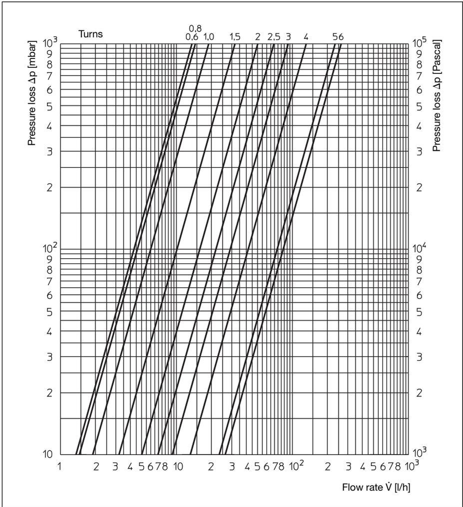
Chart 2: Pressure loss chart bypass, valve closed
