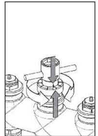
5. Setting is carried out by turning the presetting key anticlockwise (a complete turn corresponds to presetting 1 etc., maximum of 6 turns)
