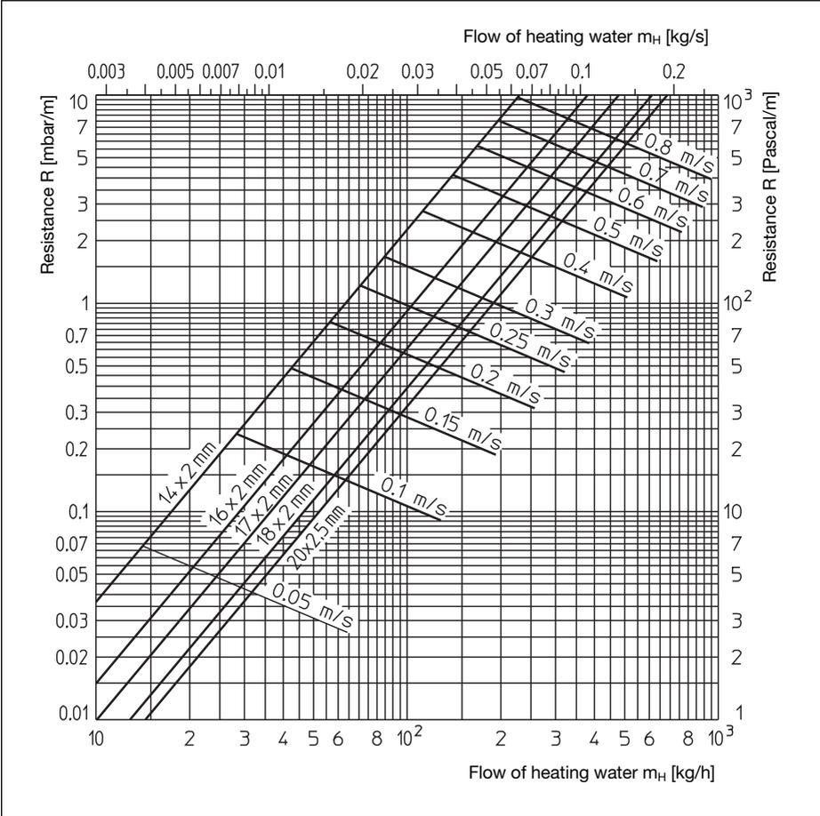
**Chart 3: Pressure loss chart for Oventrop pipes**
