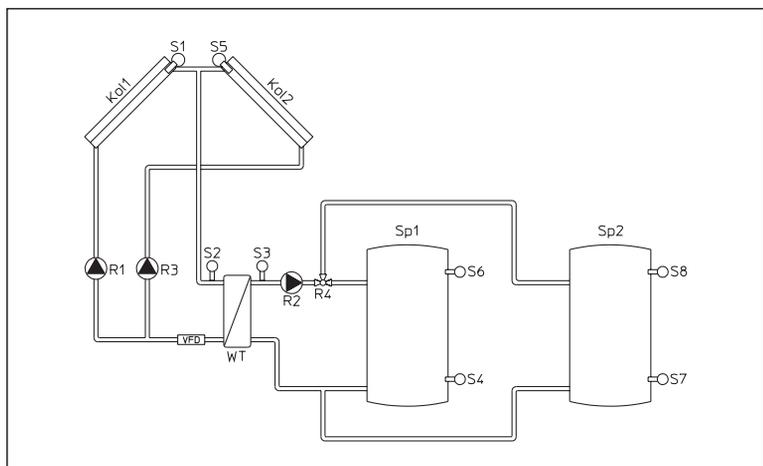
For 2 collector fields with storage cylinder connection for loading of 2 separate storage cylinders
