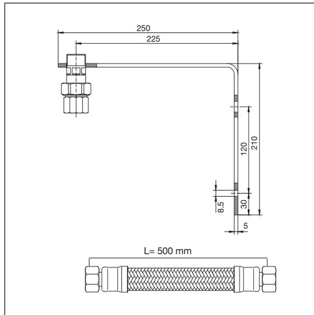
Dimensions connection set for diaphragm expansion tanks
