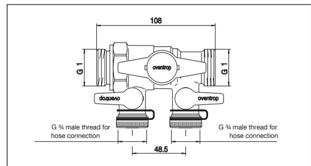
Dimensions “Regusol” filling and flushing device
