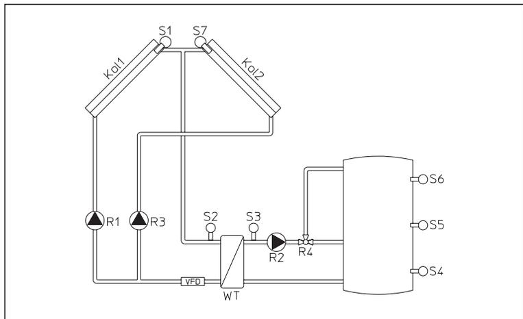
For 2 collector fields with storage cylinder connection for loading section by section
