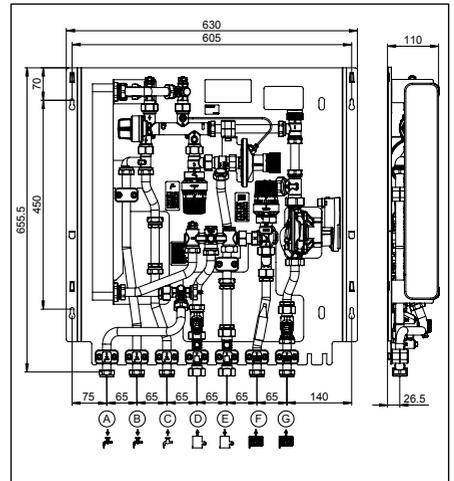
Illustr. 4.4 Dimensions with variable temperature circuit
