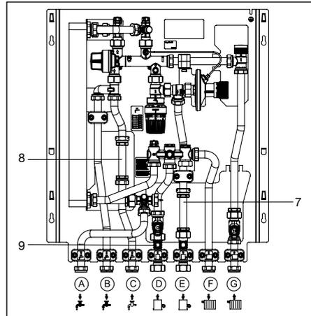
Illustr. 6.1 Installation cold water meter and heat meter
