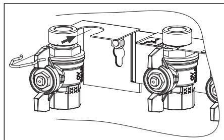
Mount the ball valve into the suspension of the connection set.
