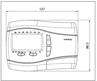
Dimensions room thermostat-clock with wireless transmitter
