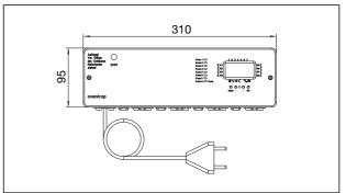
Dimensions wireless receiver with time switch, 8 channels
