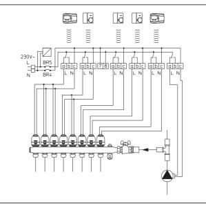
System illustration 3 with connection diagram
