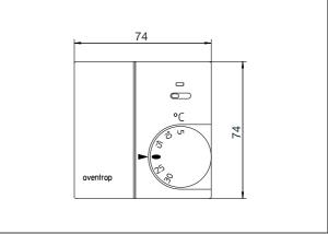
Dimensions room thermostat with wireless transmitter
