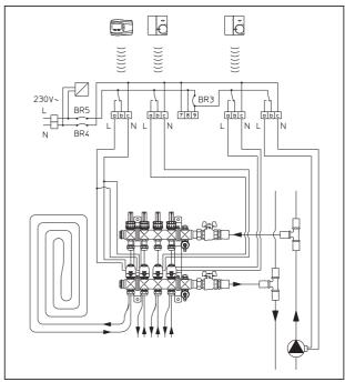
System illustration 2 with connection diagram
