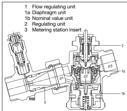
Illustr. 5.2 Construction "Cocon QTZ" with metering station
