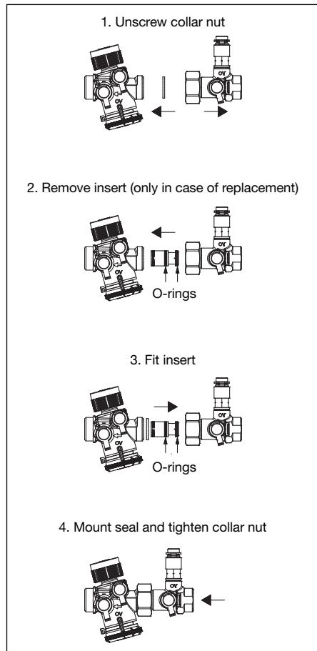
The installation direction of the insert must be observed during installation.
