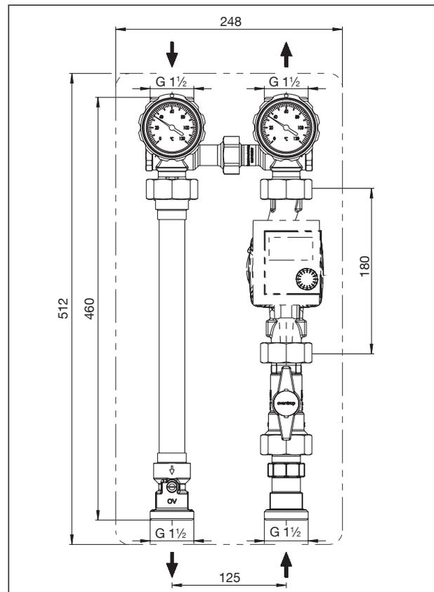
Dimensions "Regumat S-180" DN 25 with pump ball valve at the pump inlet
