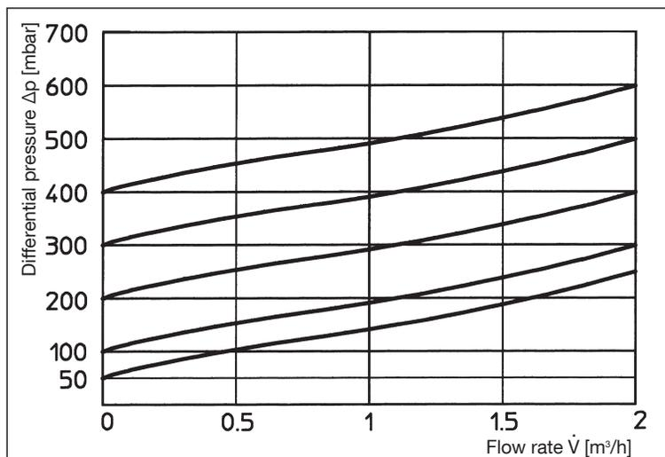
Flow chart bypass (pressure relief device)
