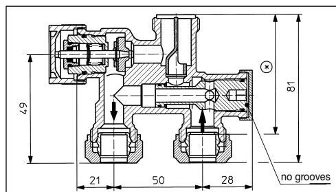
\* 66 mm for precision steel/copper pipe Ø 12 - 16 mm
