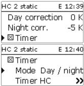
The parameter  $\boldsymbol{\mathsf{Mode}}$  is used for selecting between the following correction modes:
