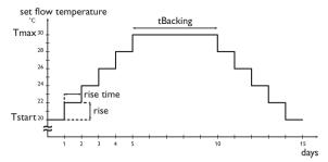
The diagram shows the parameters of the screed drying with the factory settings.
