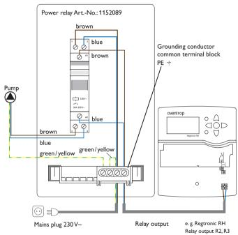
Relays 1 and 4 are electromechanical relays for loads with high current consumption. If loads with high current consumption are to be connected to relay 2 and / or 3, pay attention to the following note:
