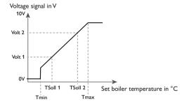
By means of the adjustment channels **Tmax** and **Tmin** the maximum and minimum limitations for the boiler set temperature can be defined.
