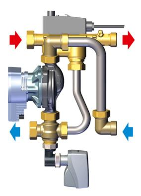
When mounting the control station to the heating circuit manifold, the correct flow direction must be ensured. The control station's supply is always at the top. Accordingly, the control station's return is always at the bottom. The control station is designed for left-hand side connection (manifold on the right, see Fig.). Righthand side connection is possible and described in the operating instructions.
