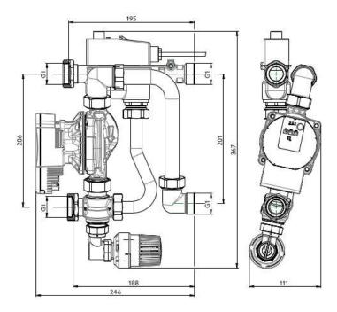
The installation depth of the control station inside the cabinet is approx. 111 mm from the front edge of the pump housing to the rear wall of the cabinet. This already includes the fastening rails.
