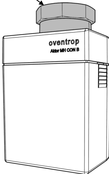
Wireless actuator “mote 320” with Collar Nut M 30 x 1,5
