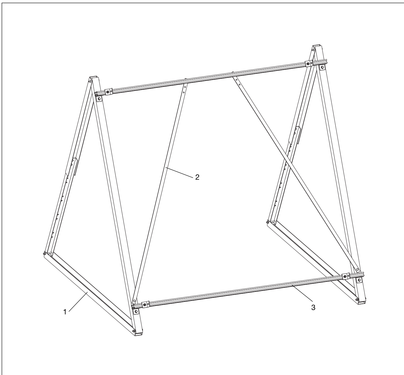
Basic set for freestanding installation item no. 1361270 and 1361275 (collectors are not included in the delivery)
