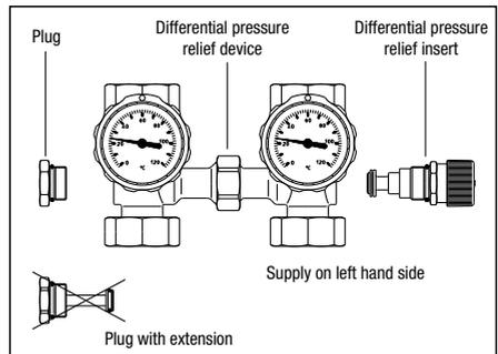
The differential pressure relief device is preset at works to an opening pressure of 200 mbar. Other opening pressures between 50 mbar and 400 mbar – to be read off the scale – can be set at the handwheel.
