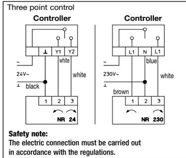
**Installation instructions for the connection to an Oventrop three-way mixing valve:**
