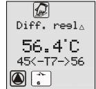
Display of the temperature of the energy source sensor in the "Information" menu, with minimum and maximum values. The corresponding measuring point – here T7 – is also displayed.
