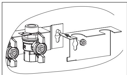
The fixing plate is fastened with the suspension of the ball valve connection set of the dwelling station onto the base plate (item no. 1341180) (use screws and nuts of the existing connection set).
