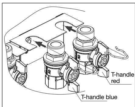
Mount the ball valves into the suspension of the connection set (position the ball valve with the red handle into the notch on the right hand side and the ball valve with the blue handle into the notch on the left hand side). Insert the enclosed locking springs below the plate to protect the ball valves.
