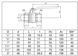
Dimensions item no. 10790.. (DN 15 up to DN 50), steel lever
