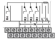
The controller is supplied with power via a mains cable. The power supply of the device must be 100 ... 240V~ (50 ... 60 Hz).
