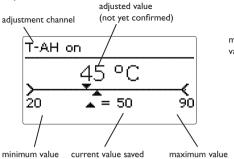
Numeric values can be adjusted by means of a slide bar. The minimum value is indicated to the left, the maximum value to the right. The large number above the slide bar indicates the current adjustment. By pressing buttons 2 or 4 the upper slide bar can be moved to the left or to the right.
