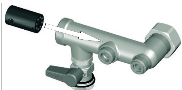
Illust. 40: Installation of the measuring turbine
