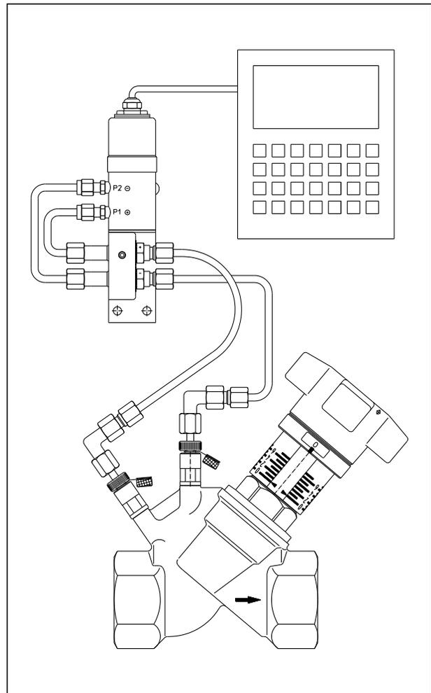
Example of installation differential pressure transmitter
