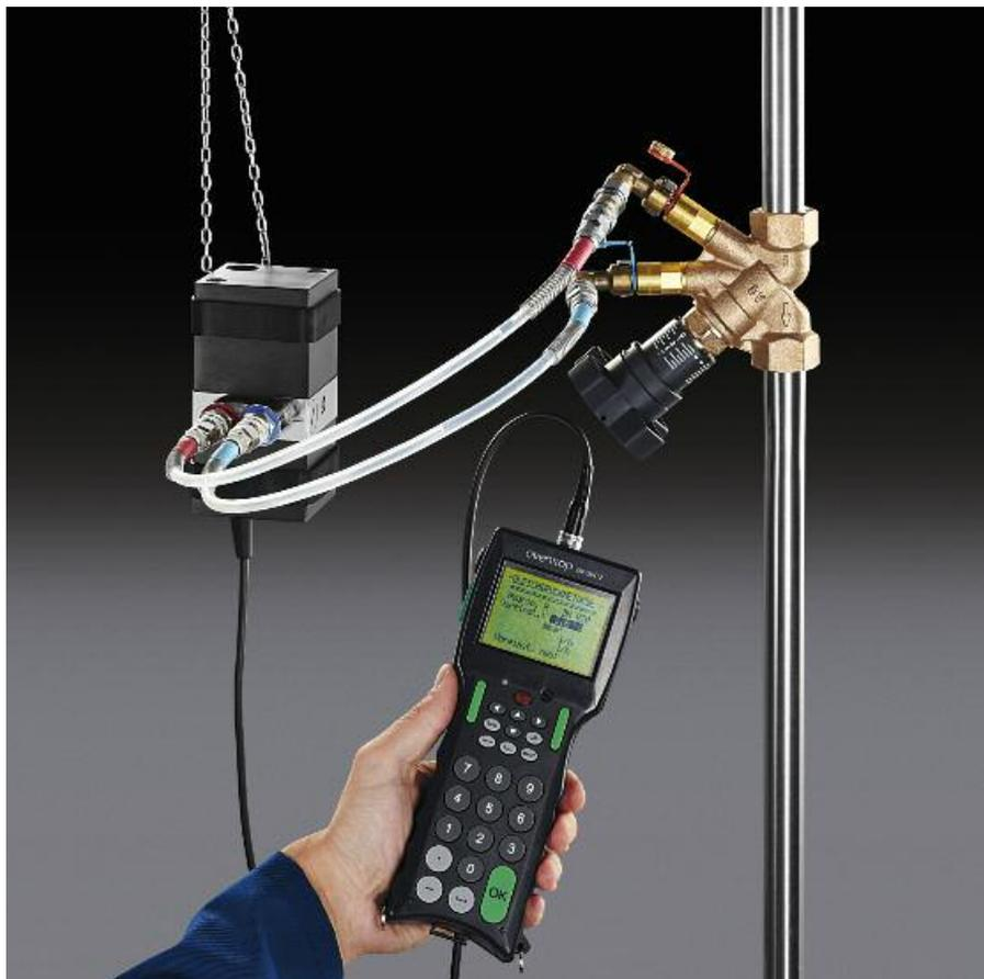
The measuring system "OV-DMC 2" was especially designed for measuring the flow of Oventrop regulating valves. It is equipped with a watertight and dustproof keyboard and has a rechargeable battery ideal for on site application.
