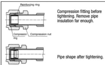
When using thin walled and very soft pipes, reinforcing sleeves have to be used. The reinforcing sleeve supports the pipe and provides the strength to enable the necessary compression. Reinforcing sleeves cannot be used on pipe with welded seams. The recommendations of the pipe manufacturers have to be observed in any case. If necessary, a practical "test" has to be carried out.
