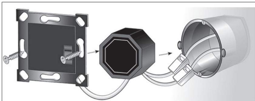
*Illust. 5: Wall attachment of the fixing plate and flush-mounted power pack*
