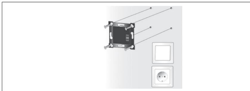
*Illust. 4: Wall attachment of the fixing plate*
