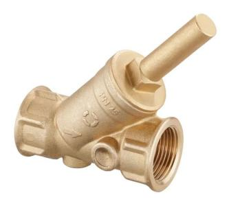
Backflow preventer made of brass for horizontal and vertical installation. Valve plug spring-loaded. For central heating and cooling systems with closed circuits and industrial plants. Not suitable for use with pulsating flow or within a distance of  $10 \times DN$  downstream of a pump.
