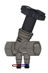
Stainless steel double regulating valve for the static hydronic balancing of pipelines in closed heating and cooling systems. The valve offers a measuring function across the valve seat. All wetted parts are made of stainless steel. The valve is available in two different material grades.
