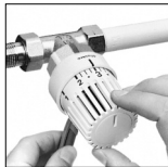
Photo 12: To remove the handgrip either the tool (item no. 1989100) or a suitable pin, e.g. the push button of a pen, should be inserted in the hole on the lower side of the thermostat. By turning the handgrip to the right into shut-off position, it is easily removed.
