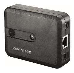
The Regtronic KM-IP communication module is used to connect the Regtronic controller to a local network for communication either via BACnet IP or Modbus TCP. It is intended for connection to a controller via S-Bus interface and for parameterisation of the connected controller, considering the specified technical data.
