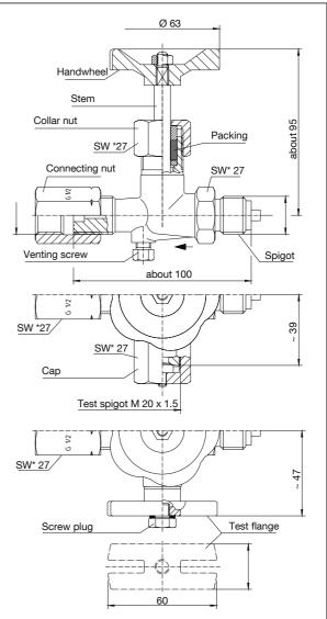
Dimensions gauge isolating valves without /with test spigot or test flange
