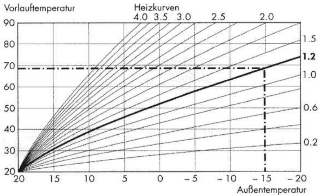
In the diagram, the "HK1.2" curve type has been selected. This means that if the desired room temperature is 20 °C and the outdoor temperature is -15 °C, then the flow temperature must be about 70 °C.
