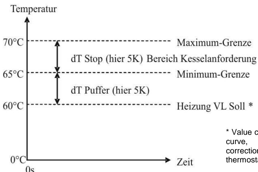
\* Value calculated from the heating curve, taking into account correction, setback and room thermostat
