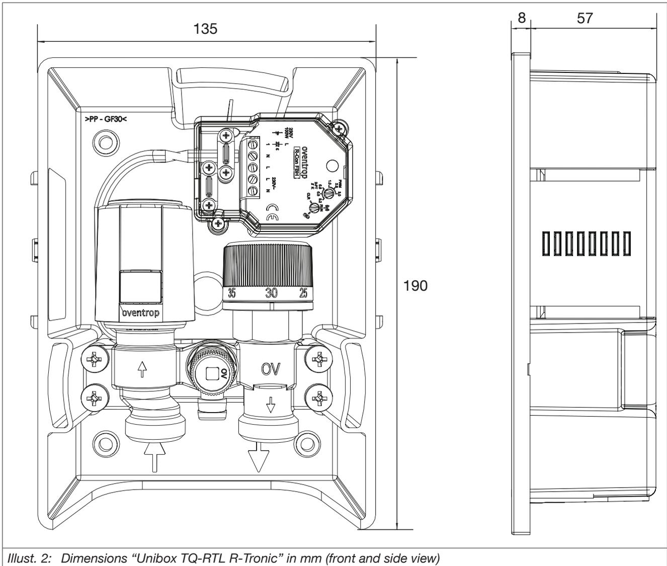
Illust. 2: Dimensions "Unibox TQ-RTL R-Tronic" in mm (front and side view)
